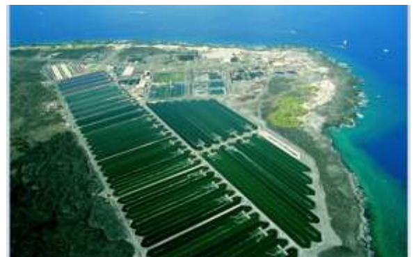
Figure 7: An ‘open pond’ algae production facility in Hawaii. Source: Cyanotech
